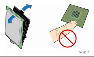
Figure 9. Remove the Processor from the Protective Cover
